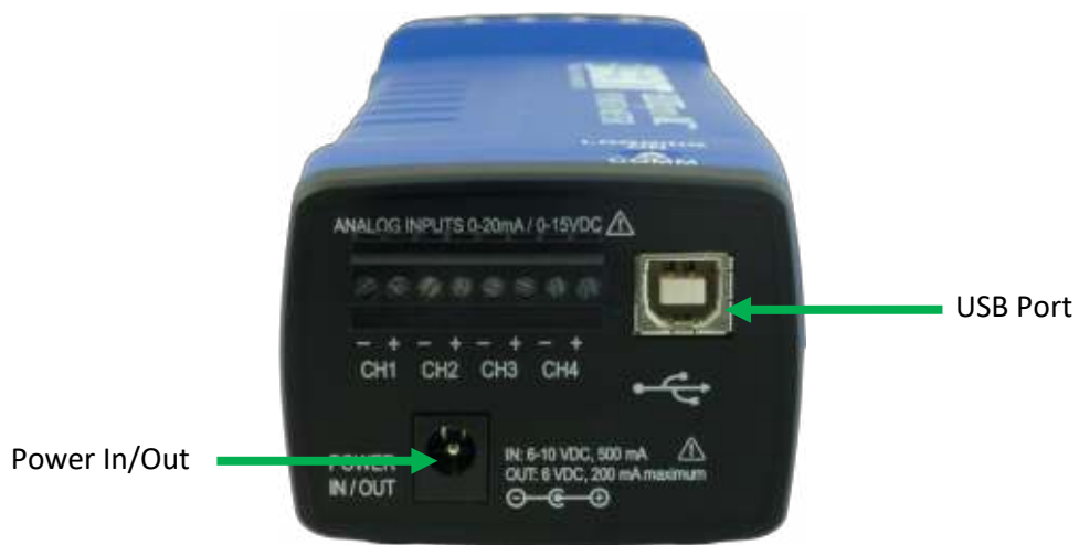
Power End Panel Connections
